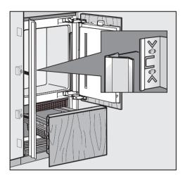
Insert the cover strip into the space between the appliance and the side panel.
